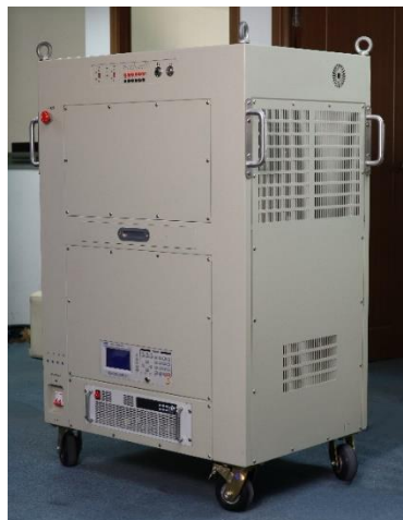
Figure 12. De-excitation switch multi-function test device physical diagram
