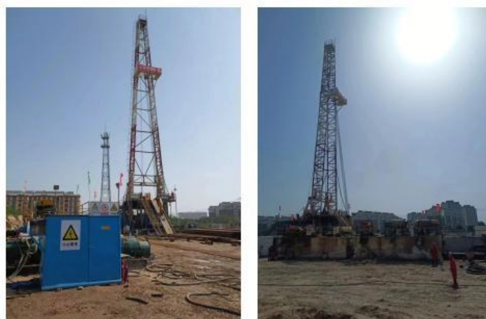
Figure 3. Drilling rig for water intake and recharge wells
