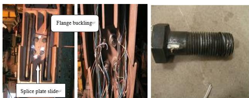
Figure 4. Failure mode of specimens
