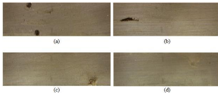
Figure 4. Image defect display of commutator cylindrical expansion (a) cylindrical slag inclusion defect (b) cylindrical imprinting defect (c) cylindrical burr defect (d) greasy dirt defect
